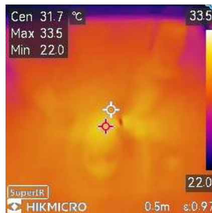
Figure 3: Nail Hole having a minimal impact to the heating up of the panel
